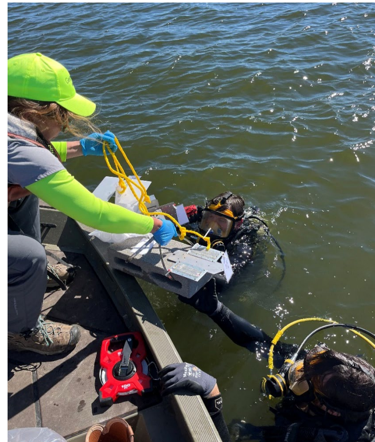
Deploying passive Surface Water Sampling Devices in Logan Martin Lake
